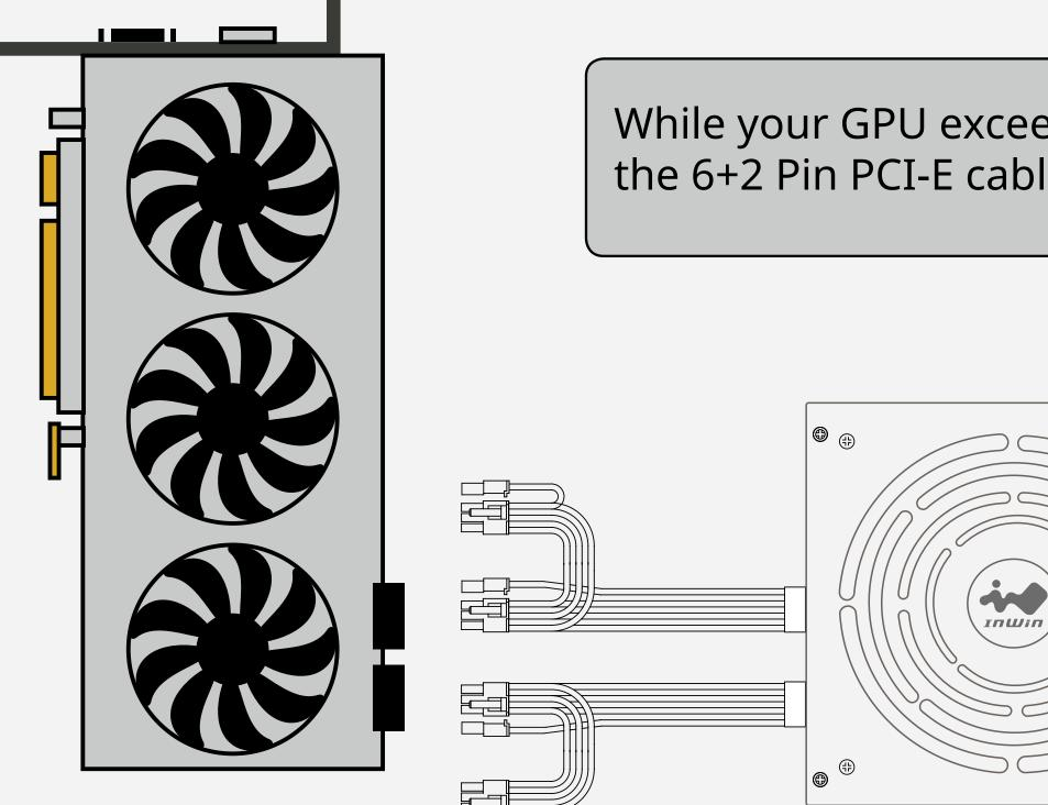
While your GPU exceeds 225W, please connect the 6+2 Pin PCI-E cables as diagram.
